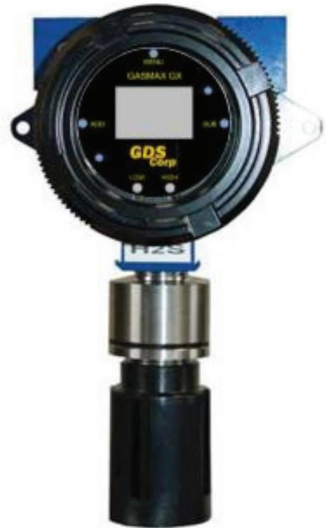
available to communicate with controllers or drive local alarm indicators. When used with the any controller's MODBUS master port, multiple GASMAX GX monitors can be daisy-chained up to 500m to minimize wiring. A special Modbus Wiring Junction Box option makes it possible to easily create the daisy chain wiring for power and Modbus signal.
