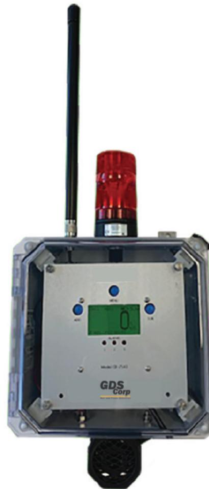
When configured with optional AC power supply, the **Protector6-RF** can supply up to 65 watts of external DC power for connected horns and strobe devices.
